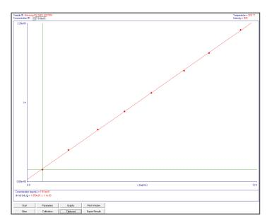
Where the dn/dc value of the sample is already known, the HK Series dn/dc differential refractometer can be used for precise and sensitive concentration determination. The amount of sample used for this can also be easily recollected and therefore utilized for further investigations.
