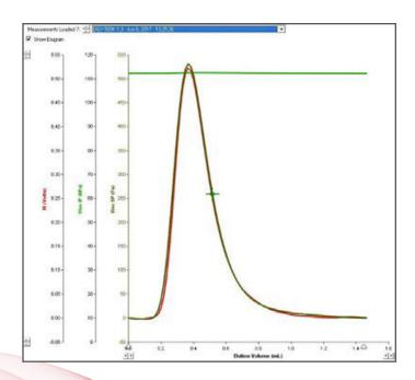
The Combo Refractometer/Viscometer sets a new standard for the detection of intrinsic viscosity of highly diluted samples. The Refractometer is an integral part of the viscometer, therefore both concentration and viscosity are measured at exactly the same time on the very same sample segment. This combination allows a much more accurate determination of molecular parameters and is particularly suited for applications focused on the structure and branching of the investigated polymer.
